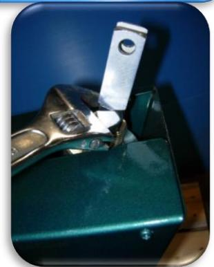
5. Reinstall the pin in place.
