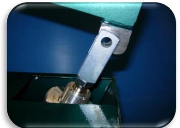
2. Unlock the nut that retained the rectangle block in place.
