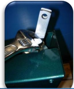
3. Unscrew the block that is screwed to the cylinder rod to adjust the height.
