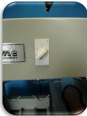
4. If you do not need to heat pieces installed on the sole rack (5) flip down the toggle switch (3). Only 4 lamps will stay on.
