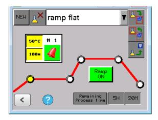
Finally button (F) need to be pressed to activate the Ramp-feature. After passing a reminder note the ramp-feature is activated and button (F) will change color from blue to green.
