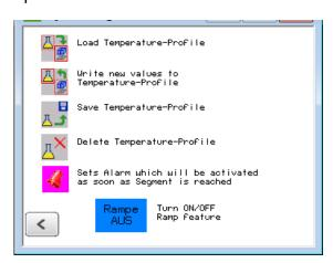
To use a heating ramp a temperature-profile must be selected from the list and loaded into the controller by use of button (A).
