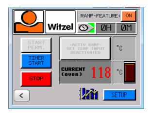
As soon as the ramp feature is activated the button for permanent oven operation as well as the set temperature input are deactivated. Both parameter are controlled by the ramp-feature resp. the Temperature-Profile of the heating-process.
