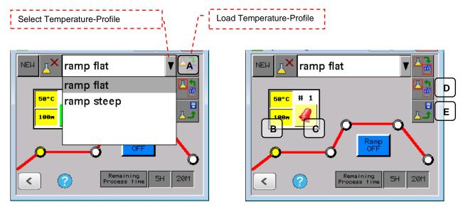
The stored values of segment 1 (yellow tap at red heating graph) will now be shown at the input mask (B). To show values of segment 2-5 the particular tap has to be activated. The values of the input mask will change to the activated segment.
